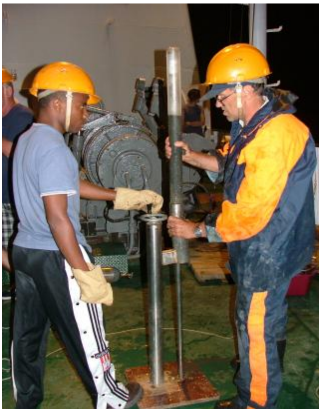
Figure 6. Prof. A. Rybalko (Russia) and Barri Ica (Guinea-Bissau) working with the Niemisto piston corer
